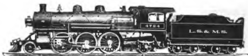
Prairie Type Passenger Locomotive Built at Brooks Works for Lake Shore & Michigan Southern Railway
